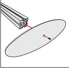
Base Plate & Extrusion Connection
