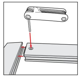
**Extrusion & Lock Connection**
